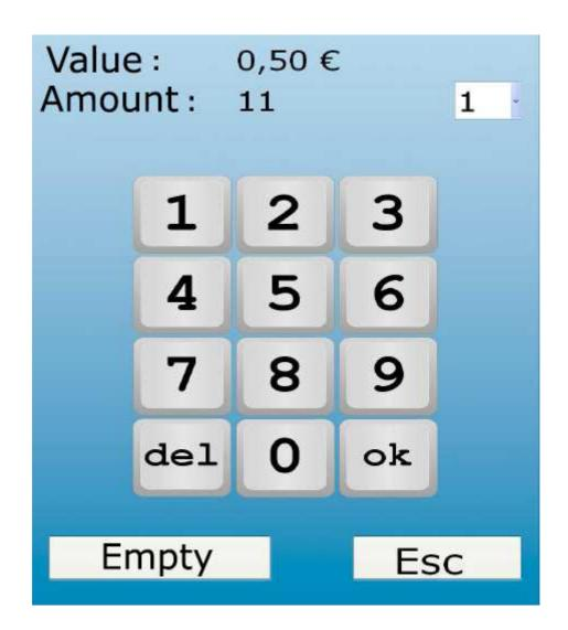
The voice "VALUE" indicates that kind of coins is present on the hopper 1. The voice "AMOUNT" indicates the number of coins present in the hopper. Always on the same line of the voice "Quantity", you will see a small window with the number 1, touching the window will open a drop down menu and you will see all the hoppers configured in the system, both coins and banknotes; selecting the 1 or 2 or 4 can do all the operations described below:
